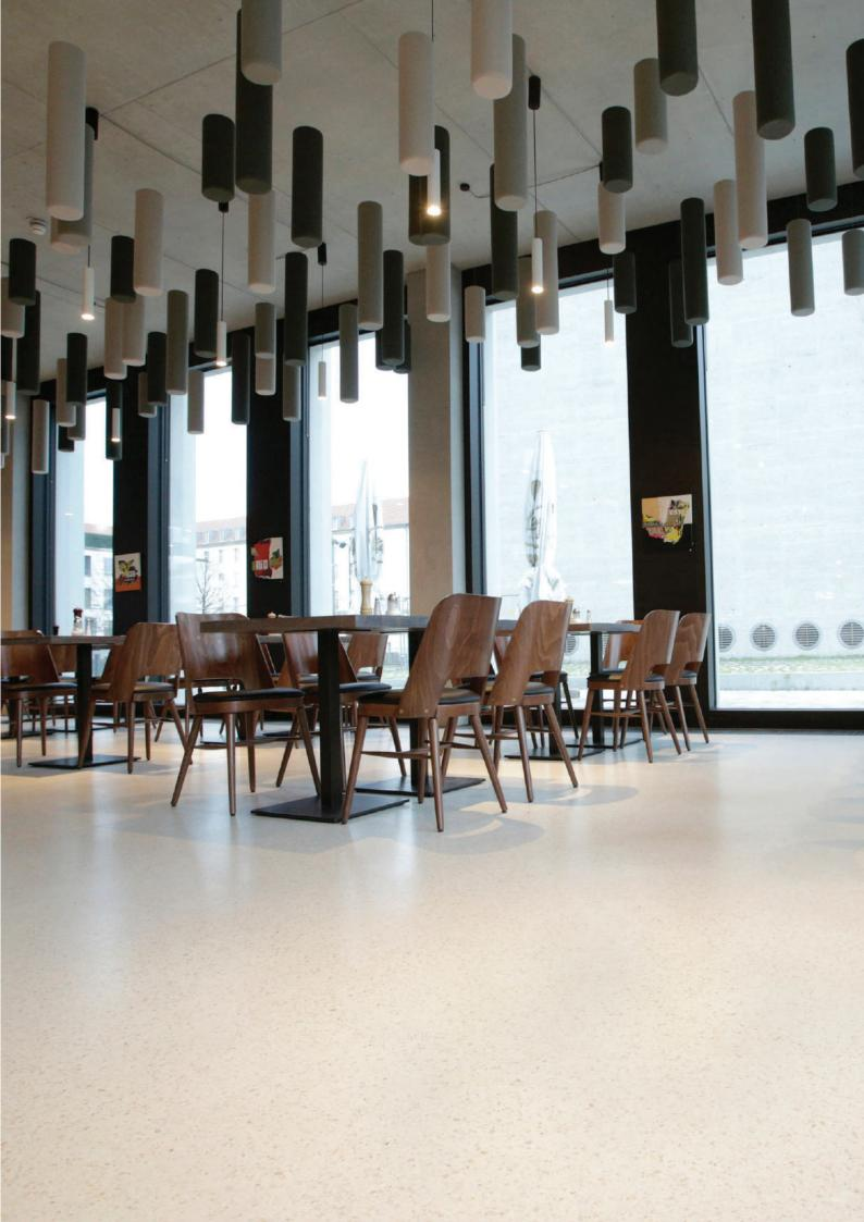
ARDEX K 390 Designer Micro-Top is a self-levelling topping with special formulated polymerised decorative surfaces. It is available in white and grey and is suitable for use in residential and commercial floor areas. ARDEX K 390 provides a smooth and level surface that can install up to a maximum thickness of 10mm in a single application. For high-stress areas, a minimum final thickness of 5mm is recommended.
